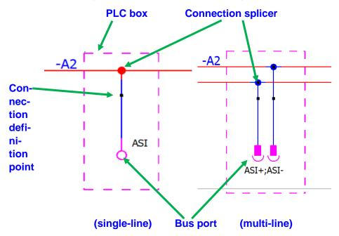
Use a symbol with fitting connection number for the multi-line representation (see chapter <u>Displaying Bus Ports in Multi-line</u> in Eplan Help).
