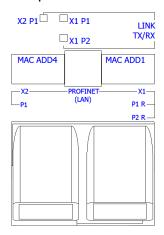
This PLC card has three bus ports for Ethernet-based bus systems:
